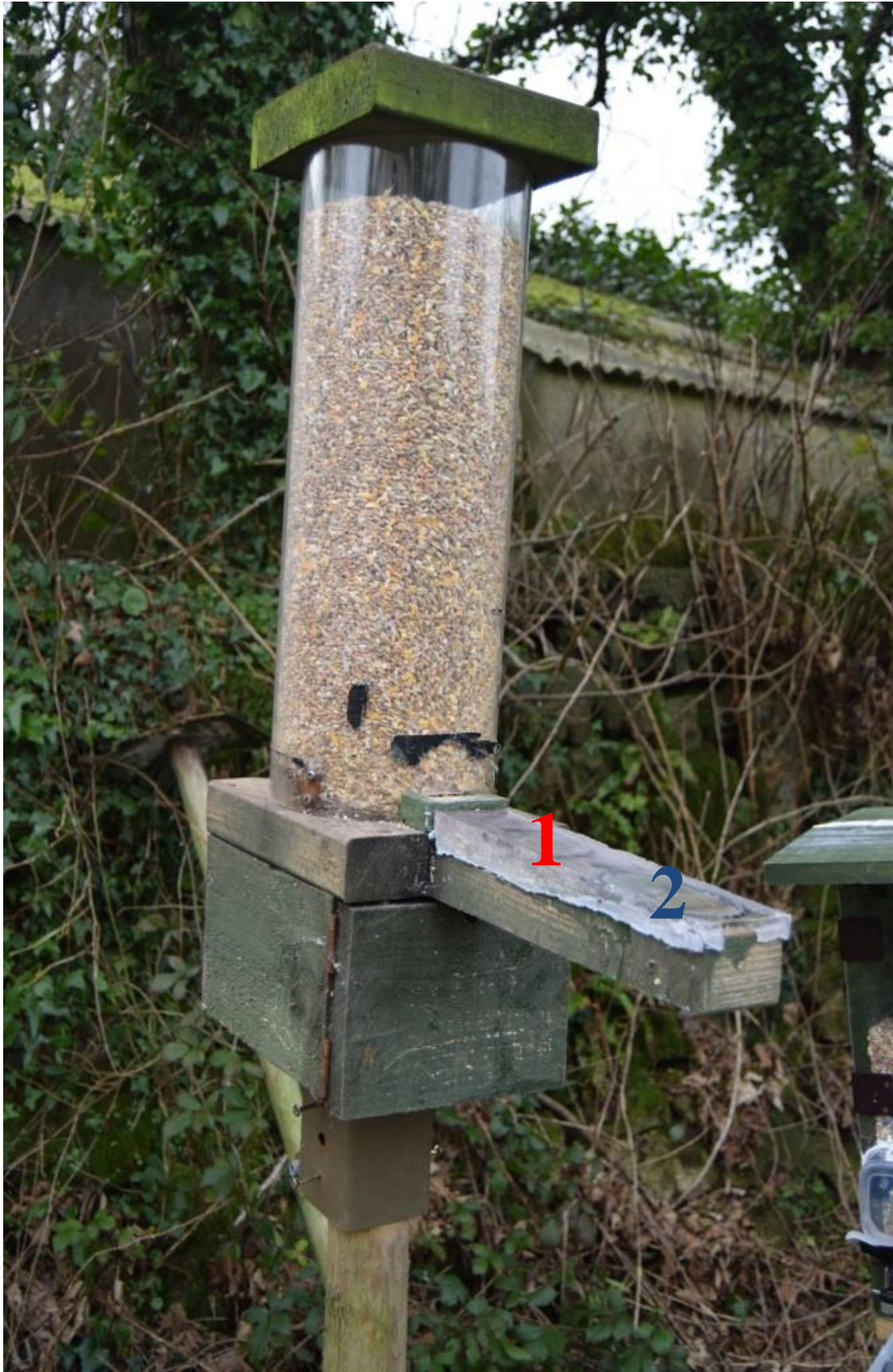
Fig. 1: Feeder equipped with an RFID reader. Two antennae are mounted on the feeding perch in primary (1) and secondary (2) positions. The feeder is filled with mixed corn.
