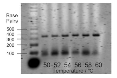
Figure 4.7: Example of agarose gel electrophoresis using a 338bp PCR product at temperatures 50-60°C. The 100bp ladder on the left enables estimation of amplicon size.
