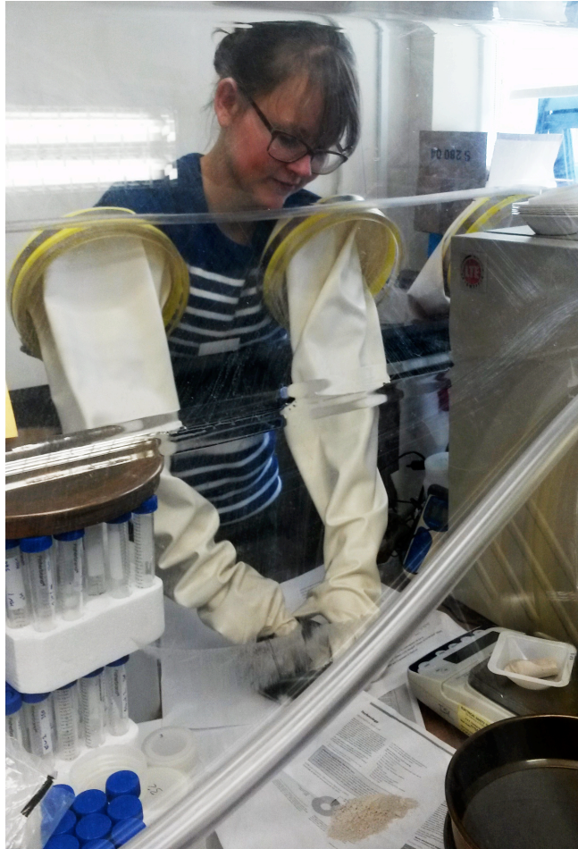
Figure 5. Doing body-work: grinding cement with a pestle and mortar in a glove box.
