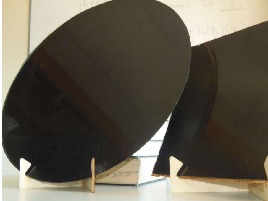
Figure 9: Spherical curvature CF prototypes with aramid honeycomb core using the 50 cm stainless steel mandrel.
