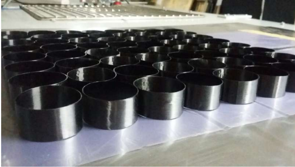
Figure 7: Carbon fiber honeycomb manufactured in our laboratory as a structural support for the mirror. This option is currently under investigation and further testing will soon be done using new molding tools.
