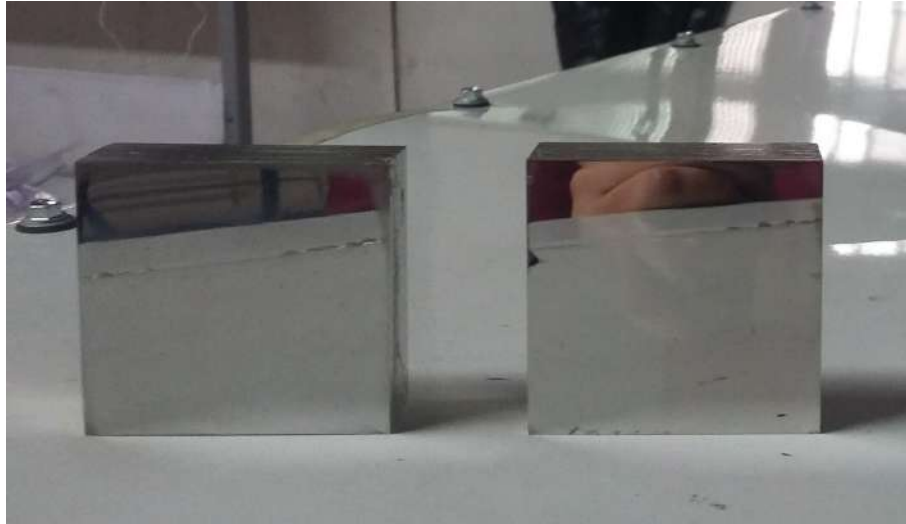
Figure 1: Polished steel mandrels used to create flat CF based prototype mirrors.
