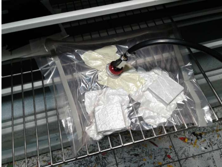
Figure 3: Vacuum bagging technique applied to small prototypes. The pressure is maintained during the whole curing process inside the oven.
