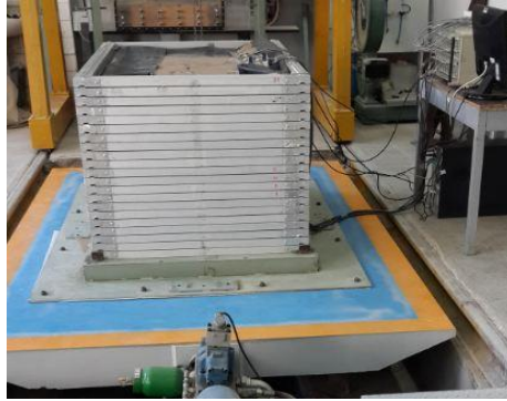
Fig. 7. Shaking table apparatus and the used shear box for experimental seismic response analysis of underground tunnel.
