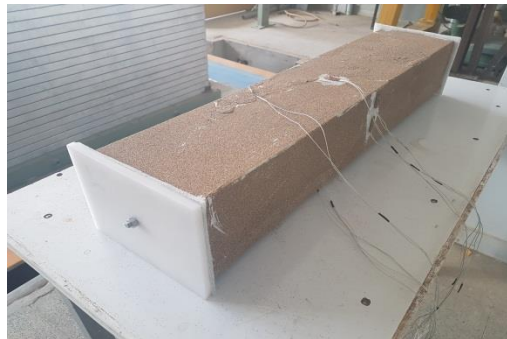
Fig. 8. The used aluminum box to model lining of tunnel
