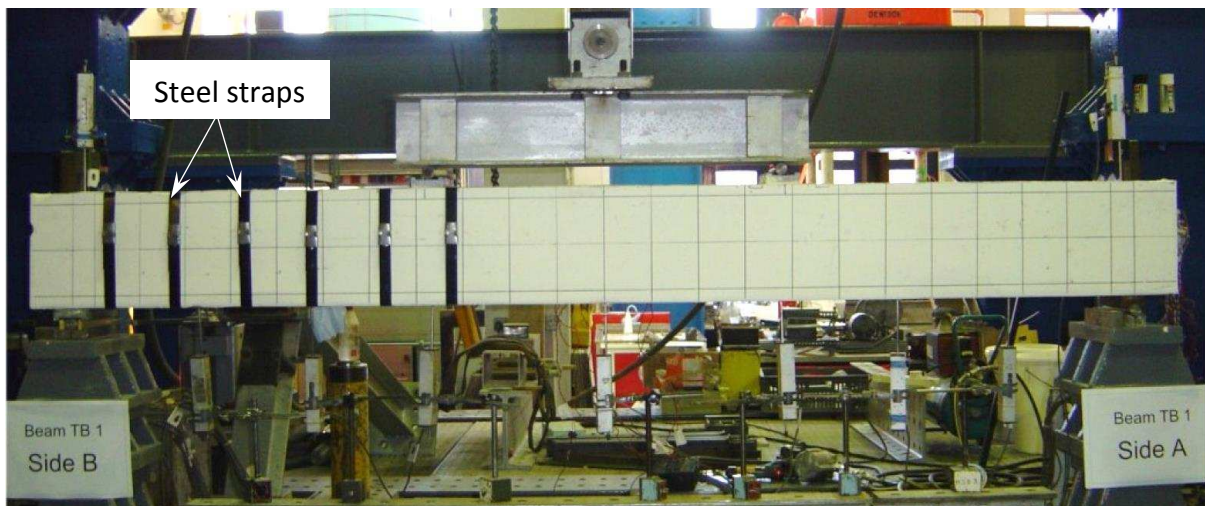
Fig. 3. Typical view of beams during tests and pre-tensioned steel straps on side B (TB 1)
