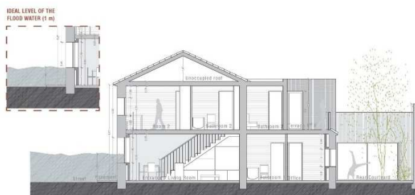
Figure 5: Long section of a single-family house with flood resistance design applied and 1 m flood water height. Source: Final MSc Thesis Project, Puchol-Salort, Jose.
