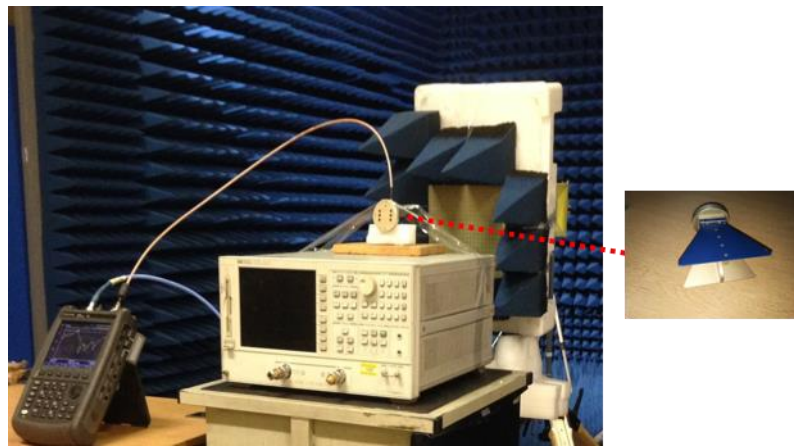
Fig. 3.19. The experimental setup to measure the transmission coefficient of the FSS.
