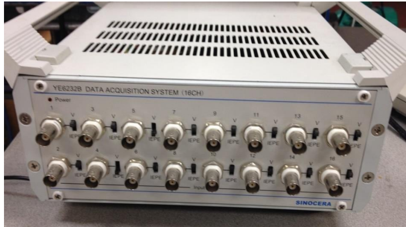
Figure 5-18 Sinocera YE6232B data acquisition system
