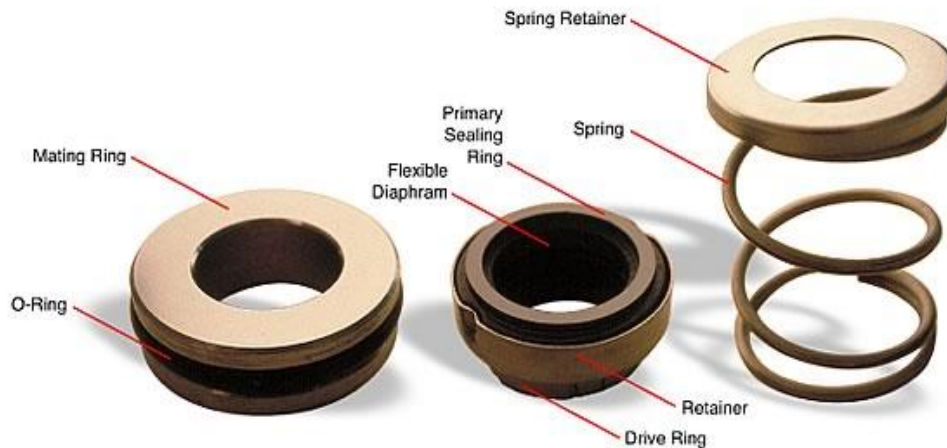
Figure 2-16 Mechanical seal [14].
