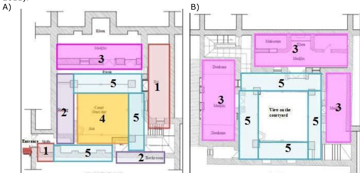
Figure 4.25: Typical layout of a courtyard house in the City of Constantine, Algeria: A) ground floor, B) first floor.
