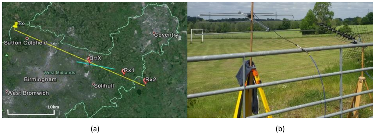
Figure 5.8. Experimental geometry (a) and receiver side in Rx1 (b) with FM and DVB-T antennas.
