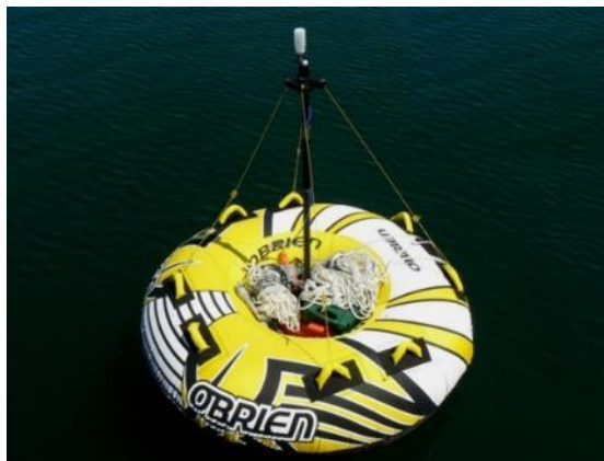
Figure 3.23. Receiver node. The Rx is installed on a ringo and equipped with omnidirectional antenna.
