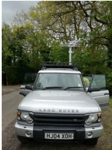
Figure 5.16. Receiver side. Rx has been installed on our laboratory car. DAB and DVB-T antennas are visible mounted on the roof of the vehicle.
