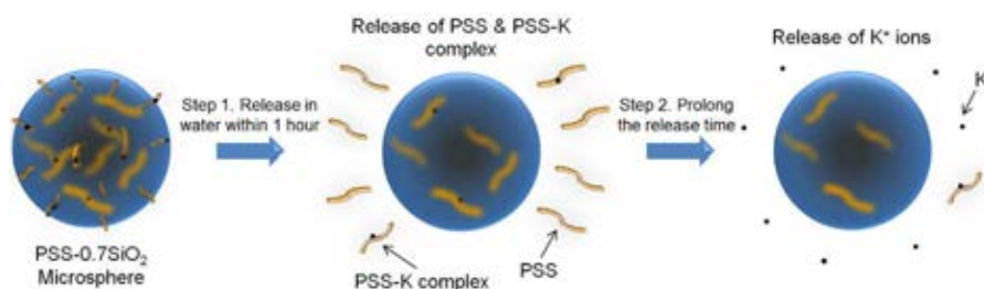
Scheme 1.2 Schematic of the ions dual-release process from the PSS-0.7SiO 2 microspheres in an aqueous environment.
