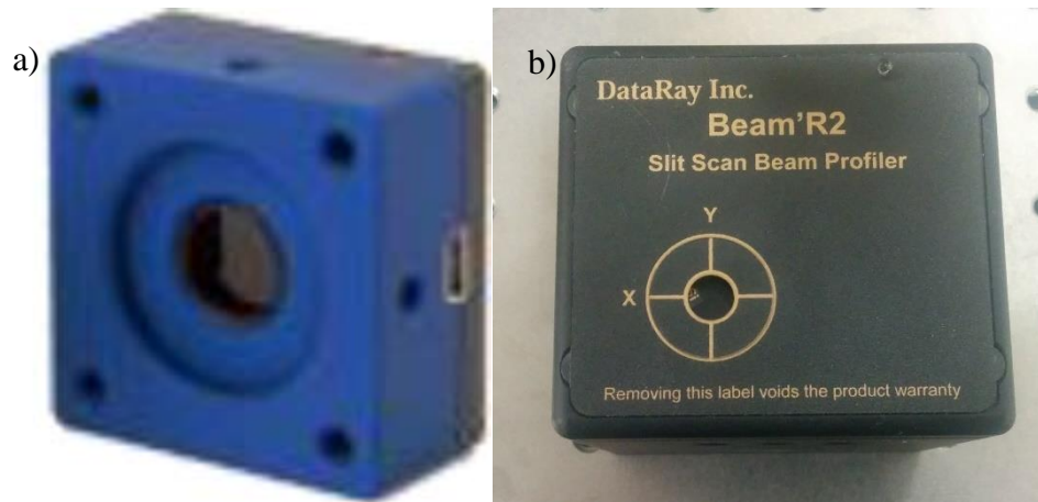
Figure 3-8 For the two-beam profile analysis, a) Camera-based and b) Slit-based devices were used
