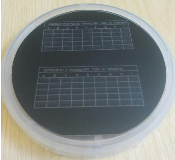
Figure 3-1 Example of a laser processed silicon wafer
