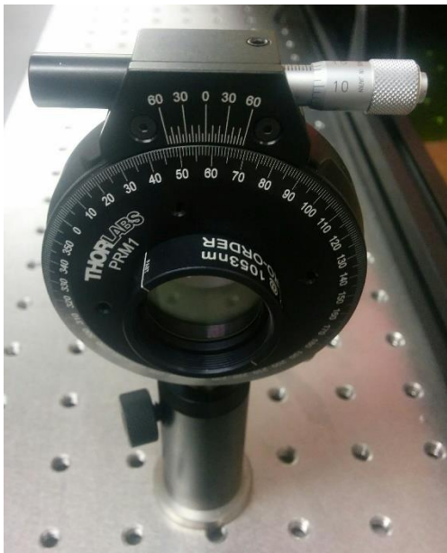
Figure 3-5 Rotation mount with a half waveplate mounted
