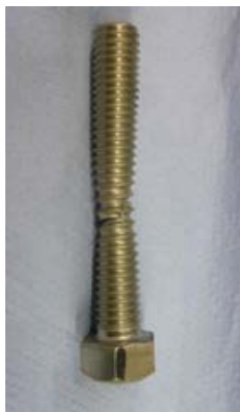
Figure 3.3 Load-elongation curve and failure mode of M16 bolt Grade A4-80 loaded in tension (Elflah et al, 2018 b)
