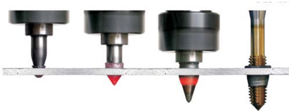
Figure 2.16 Application of the flowdrill process (Flowdrill, 2018)
