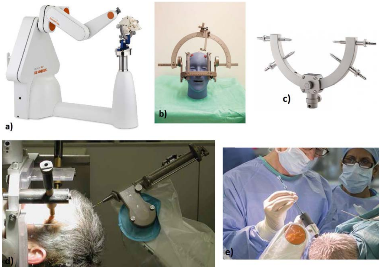
FIGURE 2.3: (a) neuromate ® with skull phantom in head holder; (b) Leksell stereotactic frame [59]; (c) head holder (Mizuho Medical Innovation) (f) patient with neuromate ® robot with drill attachment and frame, robot arm is covered with a sterile drape; (g) Insertion of a biopsy needle through a tool guide mounted on the neuromate ® arm. Except where stated, images are from Renishaw plc [60].
