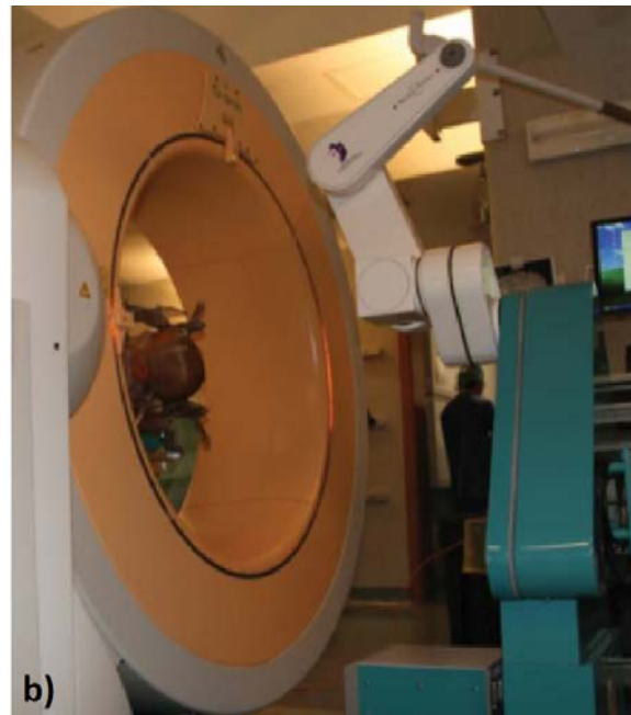
FIGURE 2.1: Calibration of robot with patient: a) calibration cage held by robot, taken from [48], originally from [49]; b) neuromate ® robot interfacing with O-arm (Meditronic), from Cardinale et al. [5]: patient's head is held in a stereotactic frame, which is attached to the robot with a frame adaptor. CT imaging allows the patient, frame and robot to be registered in theatre.
