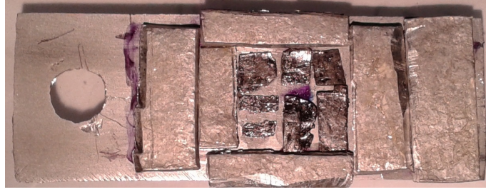
Figure 8: \text{TlNi}_2\text{Se}_2 mozaic made from 6 samples of approximately 2 mm by 3 mm surface area and 0.13 mm thickness. They are aligned with the c axis perpendicular to the mounting plate and the a and b axes co-aligned along the length and width of the mounting plate, respectively. This image is the sample setup for the preliminary measurements conducted at PSI, November 2015.
