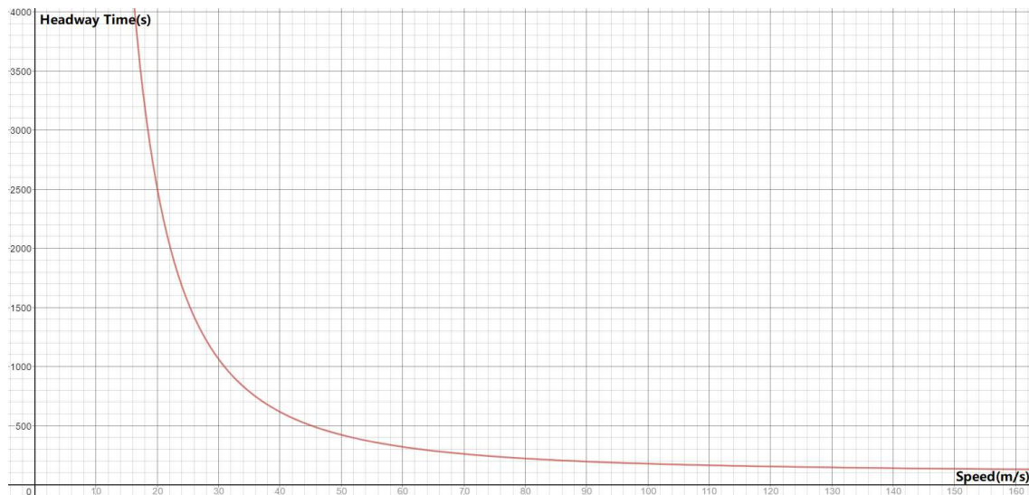
Figure 23 – Relationship between Speed and Headway Time for \Delta v = 5\text{ m/s} (Author, 2017)
