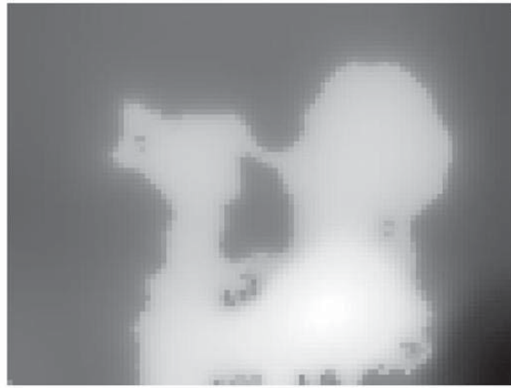
Figure 1.16: An image showing the different patch sizes used for depth based rendering. The lighter regions indicate a larger patch size (the foreground of the image) and darker regions the smaller patch sizes (background of the image)
