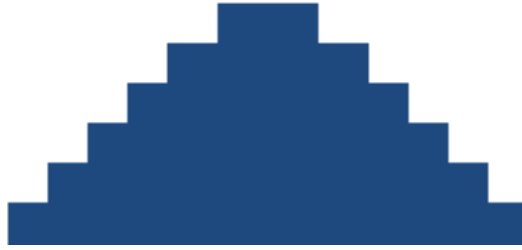
Figure 7.11: A schematic of a single microlens mould fabricated via the MSL to be used in the PMMA casting method to smooth the stepping created by MSL.
