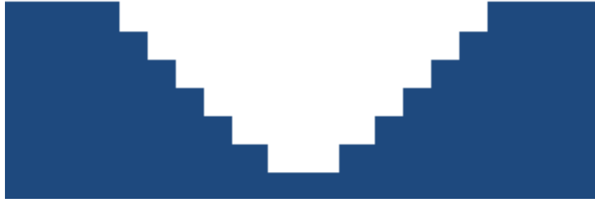
Figure 7.4: A schematic of a single microlens mould fabricated via the MSL method
