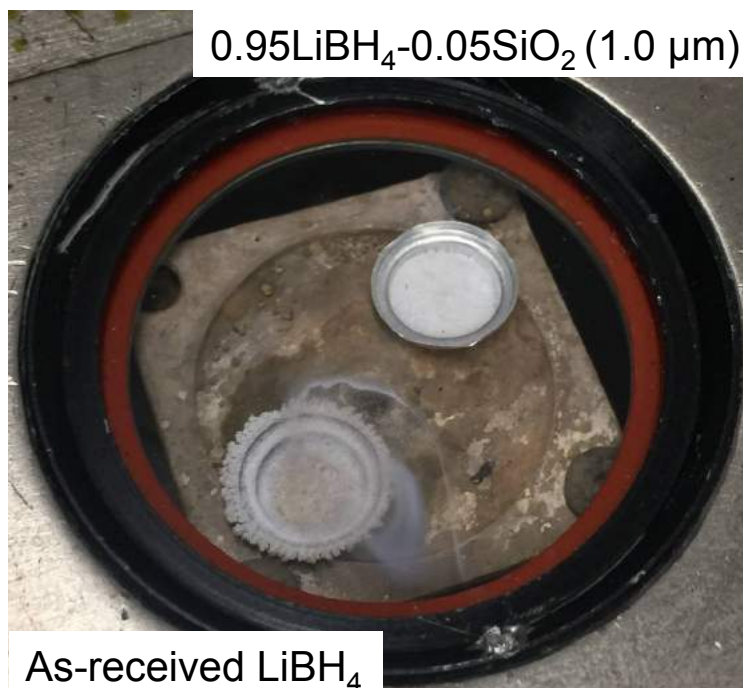
Figure 7.17 Photo of decomposed \text{LiBH}_4 sample (flake like) and 0.95\text{LiBH}_4\text{-}0.05\text{SiO}_2 sample (compact). The inner diameter of the red circle is 2.5 cm.
