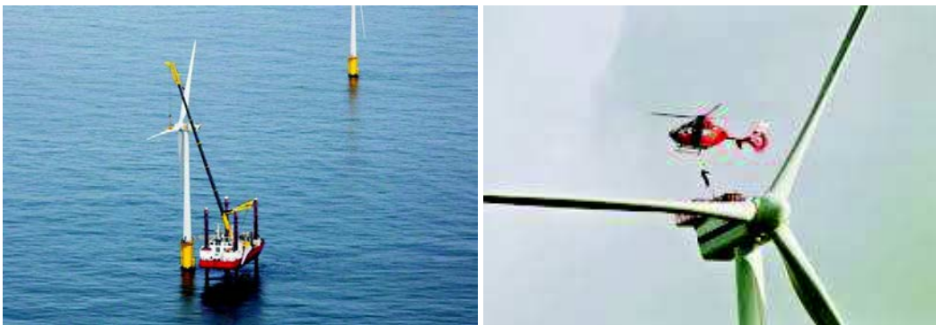
Fig. 1.5: Vessels and helicopters are used by the personnel to reach a WT.
