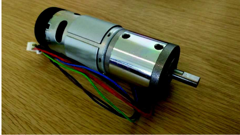
Fig. 4.6: DC motor used to set the rotational speed of the WT at a known value.
