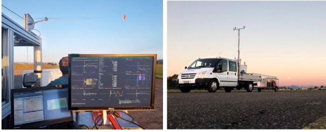
Fig. 12. The ground station, shown on the left, contains the winches, tether feed-out system, and the monitoring/control hardware. The towed configuration is shown on the right. A pole-mounted anemometer and wind vane provide wind speed and direction measurements.
