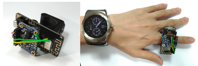
Figure 7. WRIST hardware consists of a customized smart-ring and a commodity smartwatch.
