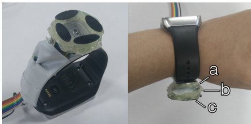
Figure 6. LensWatch allows gesture interaction on any surface, using an optical sensor mounted below the smartwatch.
