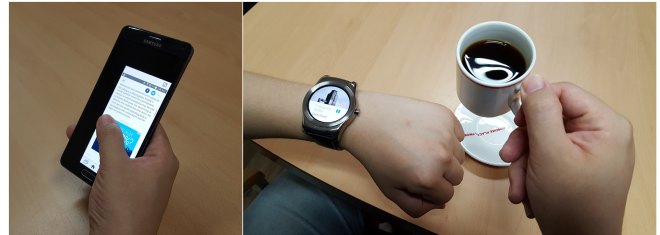
Figure 1. Example problems with single-handed interaction (left) it is difficult to reach all area of the screen with the thumb, resulting in alternative solution such as shrinking the user interface (right) it is difficult to impossible to touch the smartwatch for interaction when the second hand is occupied.
