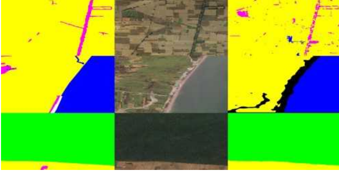
Figure 10: Remote Sensing Image Classification: The left hand side is the result from baseline approach provided by [11], the middle is the corresponding original image and the right hand side is our classification result. We apply different colors to identify different region classes as used in [11].
