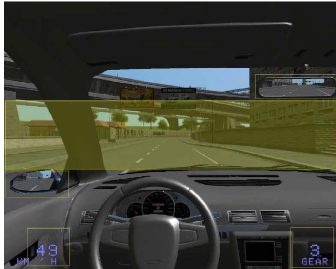
Figure 3.3. Illustration of the visual area of interest (roadway) highlighted in yellow. Screen dimensions: 1280 \times 1024 pixels ( 41.9 \times 33.4 cm; 38.5 \times 31.1 deg). Interest area dimensions: 1280 \times 266 pixels ( 41.9 \times 8.7 cm; 38.5 \times 8.3 deg).
