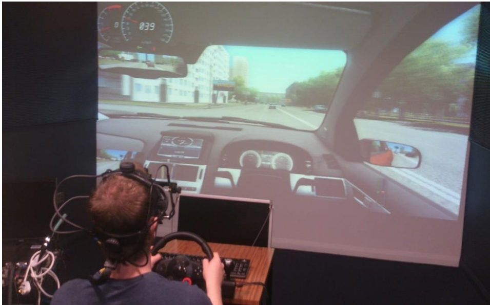
Figure 4.1. Photograph showing the basic experimental set-up. Participants sat 338cm from the projection screen. Screen dimensions: 377cm (58.3 deg) x 212cm (34.8 deg).
