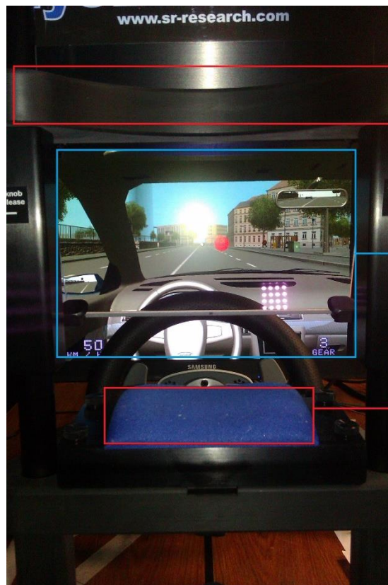
Figure 3.2. Pictures showing the eye tracking and driving set-up (a) and (b) a representation of the typical participant view point
