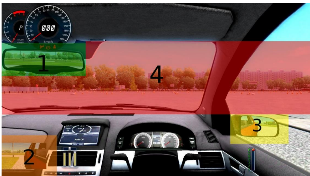
Figure 4.6. Static illustrations of each interest area. 1) Rear-view mirror (16 deg x 5 deg); 2) Passenger-side mirror (12 deg x 5 deg); 3) Driver-side mirror (19 deg x 7 deg); 4) Roadway (58 deg x 27 deg at maximum length and height).
