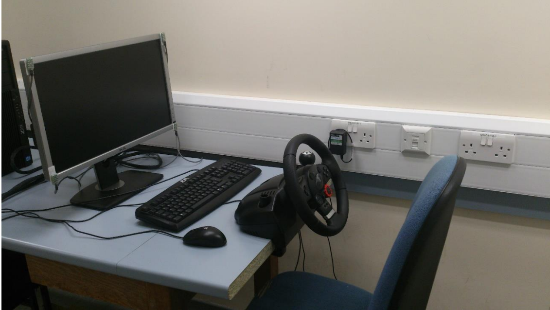
Figure 6.1. Apparatus set-up. Participants sat on the seat on the right and viewed the driving simulation on the monitor and controlled the vehicle using the steering wheel. Note, the keyboard and mouse were used by the experimenter, these were not used during the driving task.
