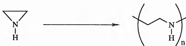
Fig. 6.6: Ring opening reaction of aziridine to produce polyethyleneamine polymer.
