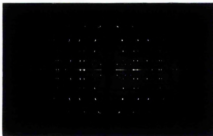
Plate 2.4: X-ray diffraction oscillation photographs, recorded at room temperature, for 1,10-dibromodecane/urea.
