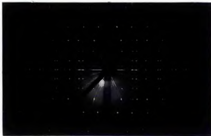
Plate 2.13: X-ray diffraction oscillation photographs, recorded at 120 K, for nonanoic anhydride/urea.
