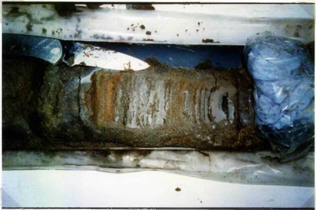
7.14 BH 80/02, from the Fetlar Basin, east central Mainland, Shetland: 7.10 - 7.30 m, knife pointing up core, showing laminated sands and clays.
