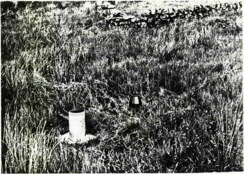
PLATE IX Black Laggan Lower rain gauge site showing the automatic gauge (foreground) and monthly crosscheck gauge in the background
