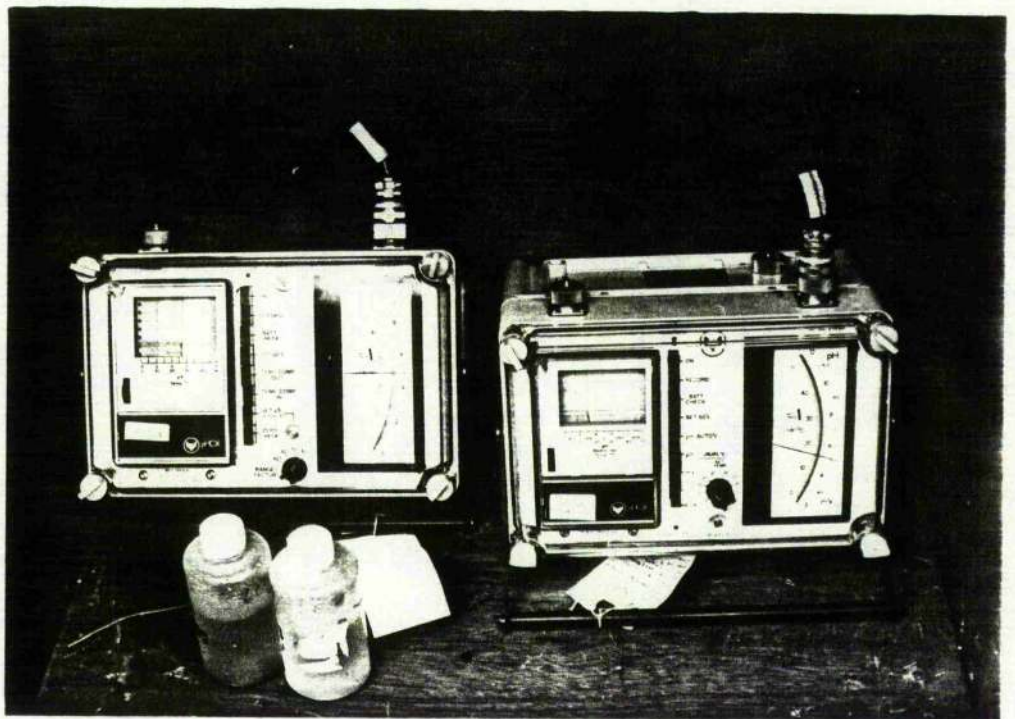
PLATE XXV The continuous water quality instrumentation common to all monitoring stations at Loch Dee
