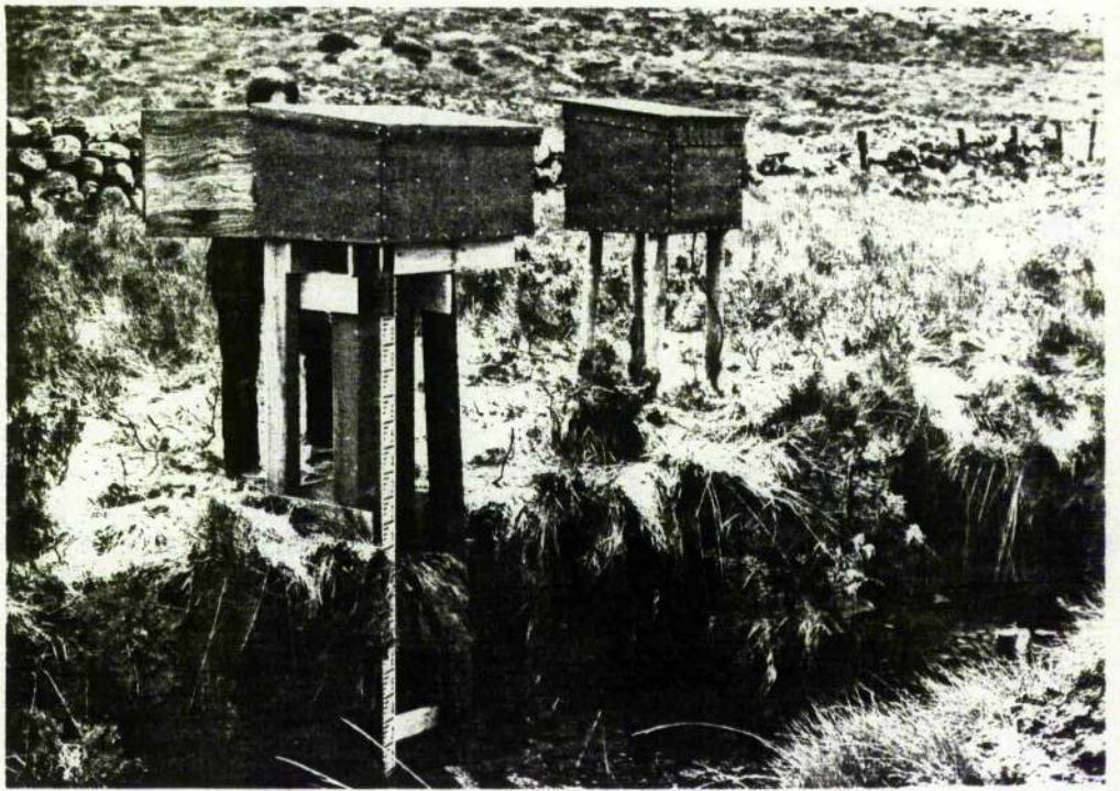
PLATE XXII The continuous water level and water quality monitoring station on Dargall Lane
