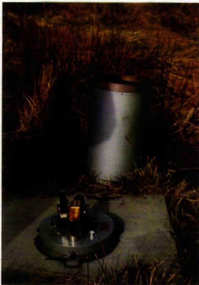
Plate 4.7: The lower autographic rainfall gauge used at Loch Dee
