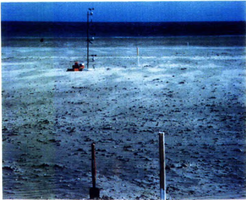
Plate 5.1 The experimental apparatus (anemometer array & traps) for measurement of sand transport rates on the beach.
