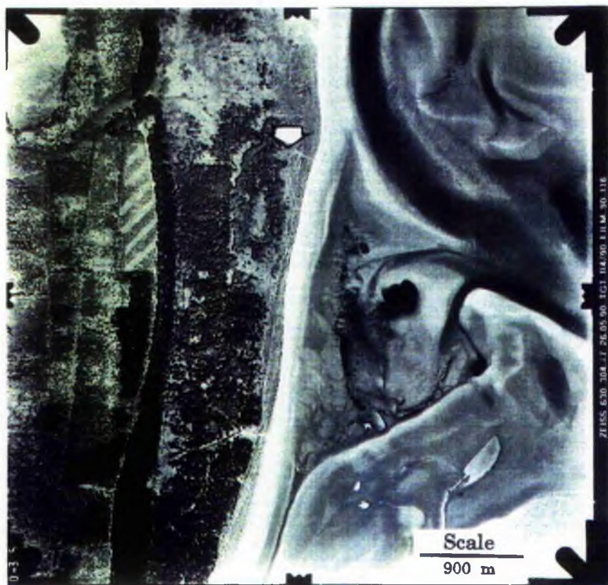
Plate 2.9 Comparison of the 1972 oblique aerial photograph with the 1990 aerial photo to show the magnitude of erosion opposite the M.O.D. arrow mark in Zone 2 (Fig. 2.3) along the Tentsmuir shoreline. Arrow mark shows the position of the observation tower. 'm' is the M.O.D. arrow mark in 1972 aerial and is not visible on the 1990 aerial photograph due to the dense vegetation canopy.
