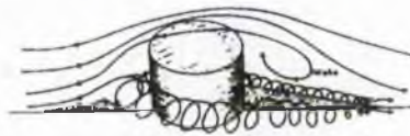
Fig. 7.5 Schematic diagram showing the development of a horseshoe vortex around an obstacle (from Pye & Tsoar, 1990).
