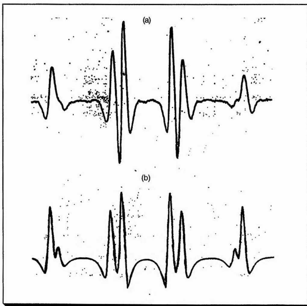
Figure 2. 36: Experimental and simulated 9.3 GHz ESR spectra of spin adducts from DMPO and S -nitrosothiol 2 in acetonitrile: (a) experimental spectrum at 298 K (b) simulation of spectra using the parameters given in the table. ESR spectra were recorded on a BRUKER ER 200 D spectrometer.
