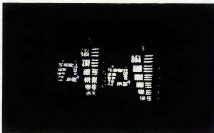
Figure 4.11.X-ray double frame result using the Picoframe II camera, first frame right, second left.
