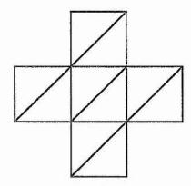
triangles are removed one by one from the outside of the shape, so that for every vertex and face, two edges are removed, again keeping V-E+F constant. Finally, one triangle remains, such that V-E+F=1, and adding the original face of the cube which was removed leads to the Descartes-Euler formula, V-E+F=2.
