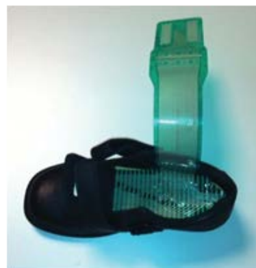
Figure 1: The F-Scan system was carefully trimmed to fit the entire plantar surface of the standardised footwear
