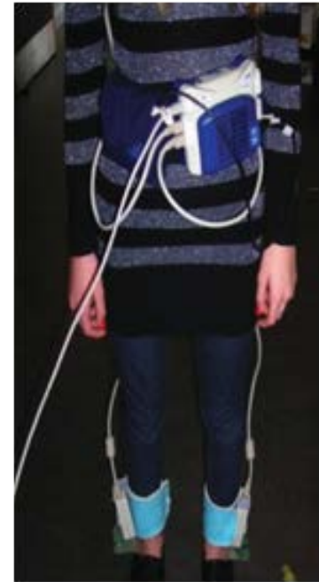
Figure 3: Represents how each participant was set up with the F-Scan system prior to each calibration and recording
