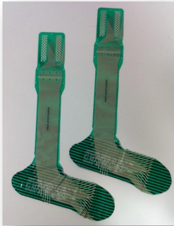
Figure 3.3.3.3: a pair F-scan insole used in the study
