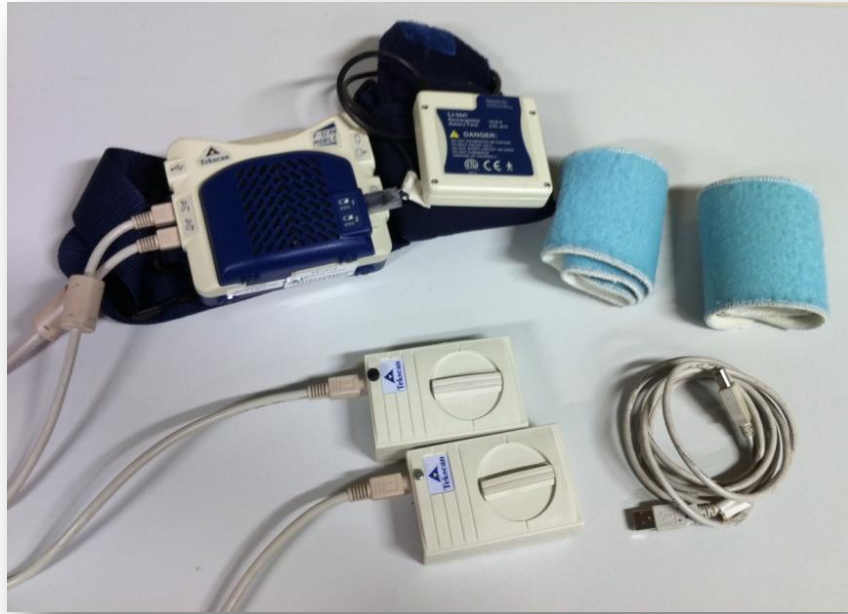
Figure 3.3.3.10: F-scan mobile unit with battery, cable, ankle cuff and strapping
