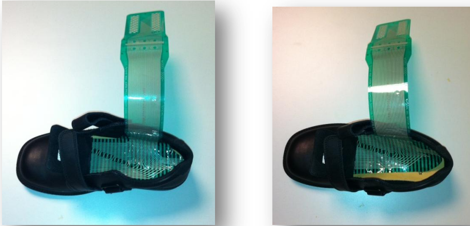
Figure 3.3.3.13: correct (left) and incorrect (right) position of the F-scan insole
