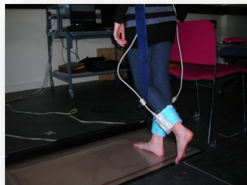
Figure 3.4.4.2: HR Walkway standing calibration with patient while wearing the F-Scan mobile unit
