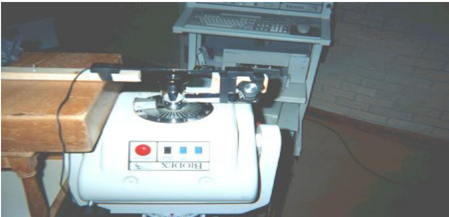
Figure 10.16: Test set-up for dynamic response of fibreoptic electrogoniometer when attached to a Biomed isokinetic unit.
