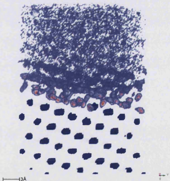
Figure 4.14: 3-dimensional projection of the structure of water above an obtuse-acute kinked calcite surface. Dark blue indicates a calcium ion, red indicates high water density and pale purple indicates low water density
