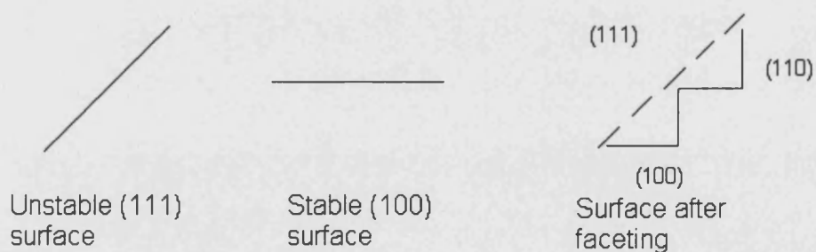
Figure 3.5: Schematic of how a faceting surface copes with polar surfaces
