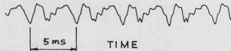
FIG. 8.7 GEAR PUMP B OUTLET PRESSURE RIPPLE BEFORE AND AFTER MODIFICATION WITH MKII MECHANISM
