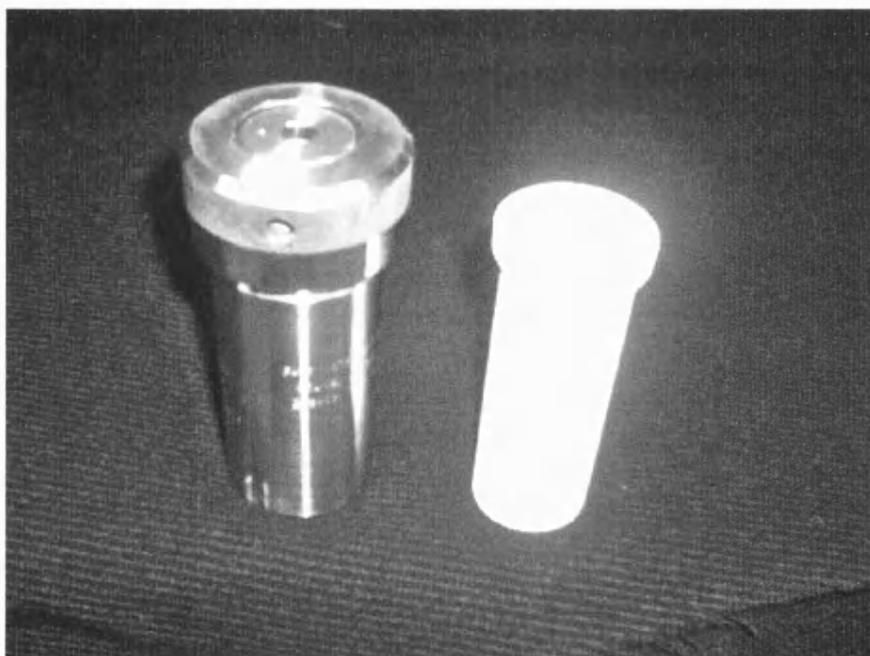
**Figure 4.1** *The PTFE lined titanium autoclaving system.*
