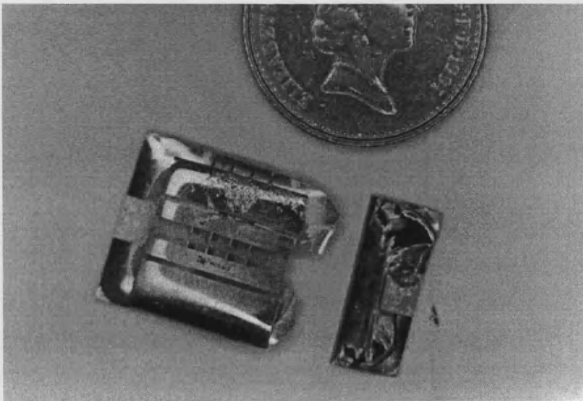
Figure 5.3. Silicon substrate (thickness 400 \mu\text{m} ) fractured beneath SU8 following copper sputter-coating (SU8 exhibited fine fracture lines over most of its surface).
