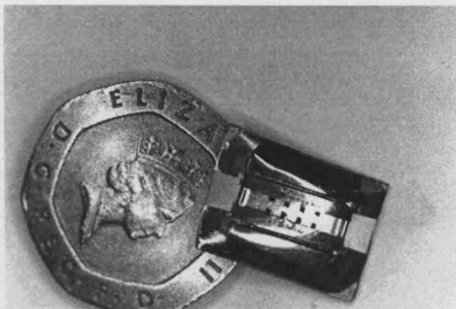
Figure 4.36. 135GHz bandpass filter (lid off) coated in nickel (multiple evaporations)
