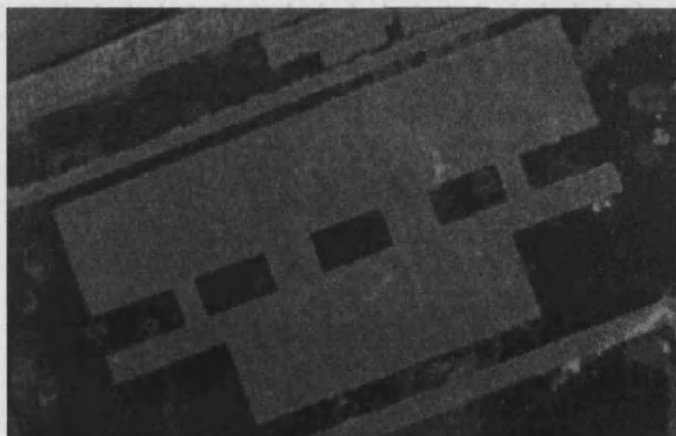
Figure 4.40. Septa foil prior to release from AZ4533 spun onto glass cover slip.
