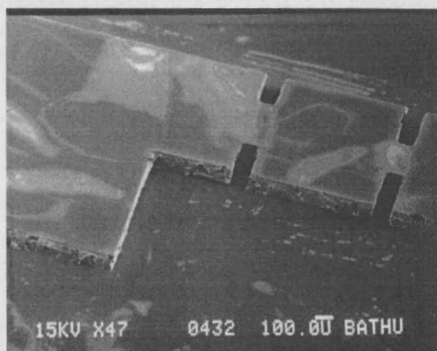
Figure 4.29. AZ4533 photoresist former (thickness 200 \mu m) for frequency doubler with activation layer (sputtered gold) for electroless plating (see Appendix 3).
