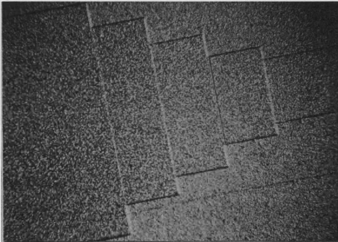
Figure 4.9. Plated resist former with height steps 20-36-48-64-80 \mu\text{m} implemented with photo-reduced greyscale mask.
