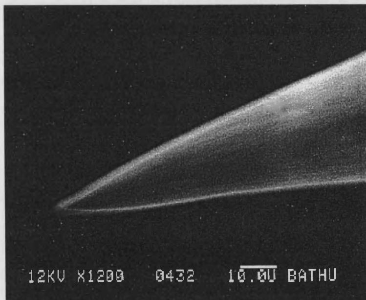
Figure 4.20. 50 \mu m diameter phosphor bronze wire with electrochemically etched tip.
