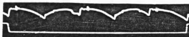
Fig 6 Measured torque and cylinder pressure at 9.2 rev/min for one half of a shaft revolution
