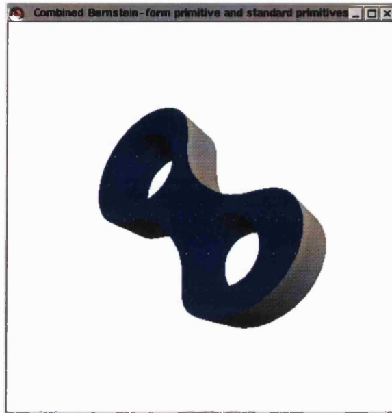
Figure 9.13: This bicycle chain link is generated by sVLIs. The grey bone-shaped object is a Bernstein-form primitive which is combined with sVLIs standard cylinder and plane primitives by using Boolean operators.
