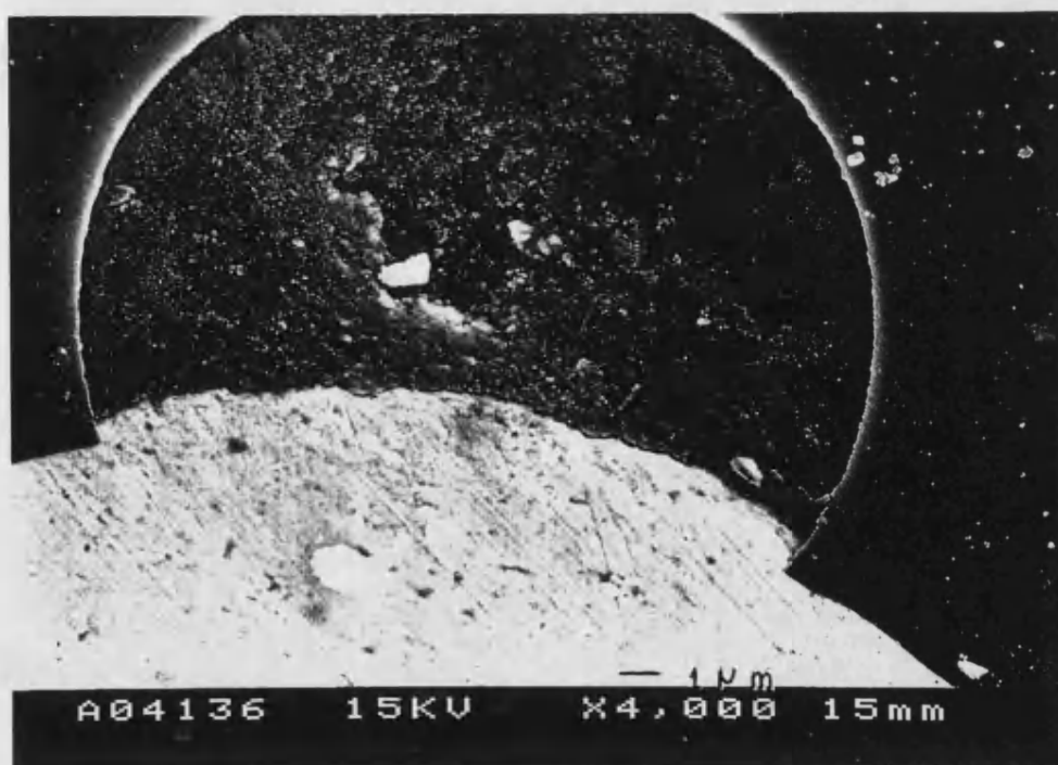
Figure 2.21b. gold-glass interface of a gold microelectrode prepared using a gold wire (60 \mu\text{m} diameter), showing bubble formation
