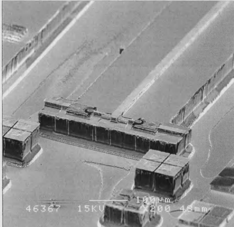
Fig. 8.5 SEM photograph showing the 45 µm deep T-etch defining the membrane outline of the finished multiplier circuit.
