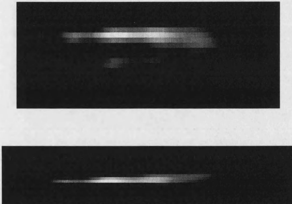
Figure 7.14. Abnormal RLE images of hot spots created on the surface of a greyed molybdenum sample.
