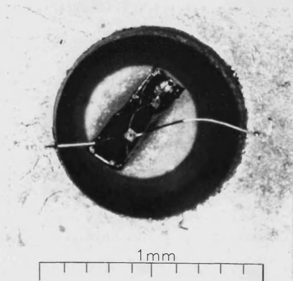
Figure III.4. An RTD chip mounted in an E3 microwave package - top cover removed.
