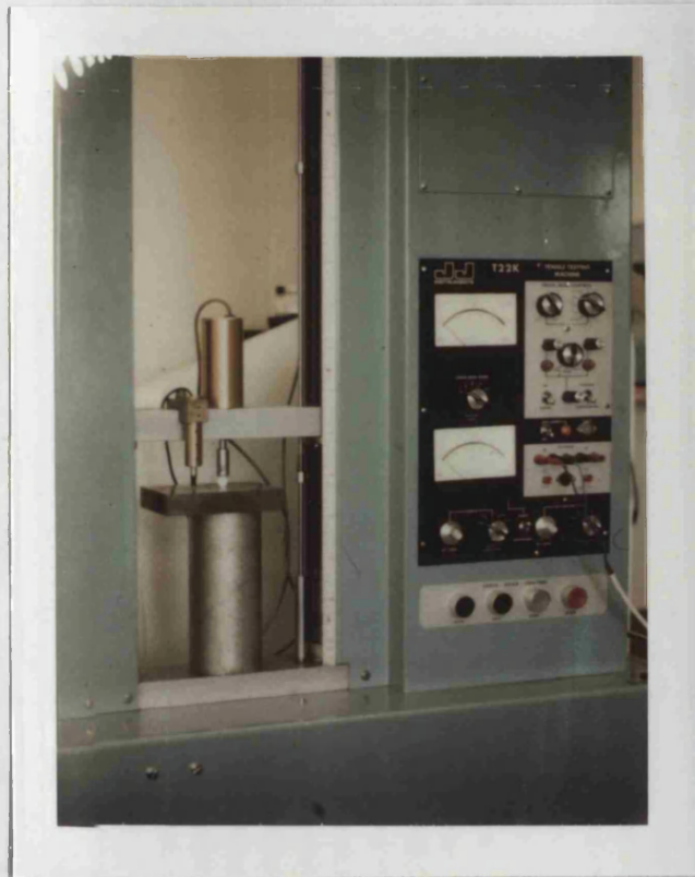
Figure 26. JJ Lloyd tensile tester with a LVDT attached to determine tablet deformation during diametral testing of tablets.
