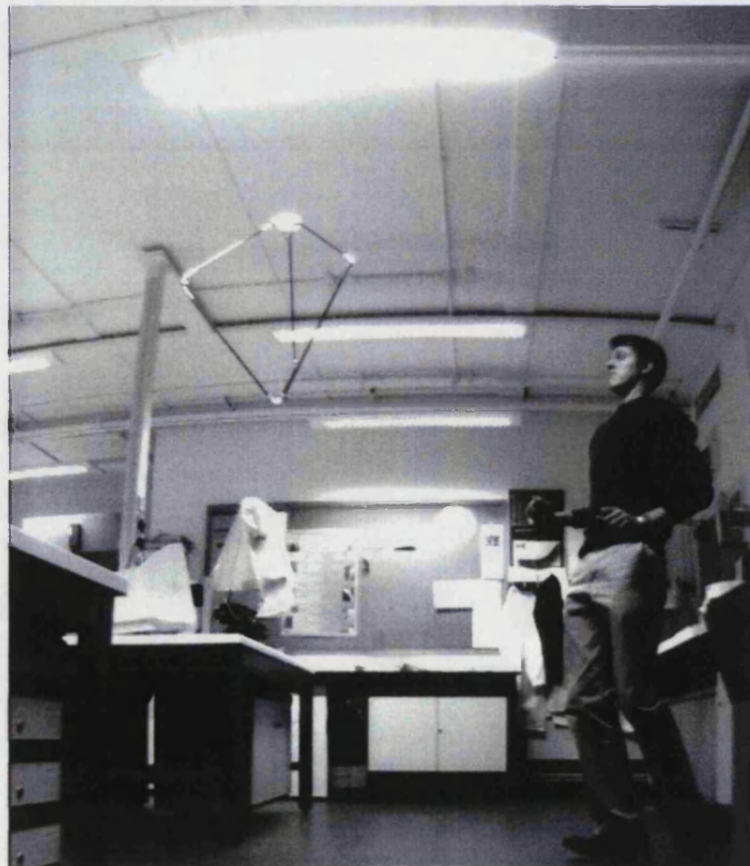
Fig. 97 – The third jumping prototype in action, taken with the high-speed camera. The base of the mechanism clears a height of approximately 1.5 m when manually released.
