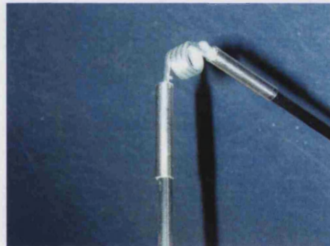
Fig. 96 – Crude sketch of the third prototype and a photograph of the reinforced carbon fibre-rods connected by a torsion spring
