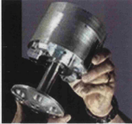
Fig. 31 – Photo of the working part of the Sandia hopper. This is mounted in a hemispherical shell which is weighted like a Weeble® toy to ensure that the piston always fires downwards for jumping.
