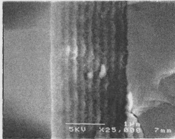
Figure 2.8: SEM image of sample C139, a 20 layer mirror formed from p- doped material. The wafer surface is on the left hand side of the image. [57].
