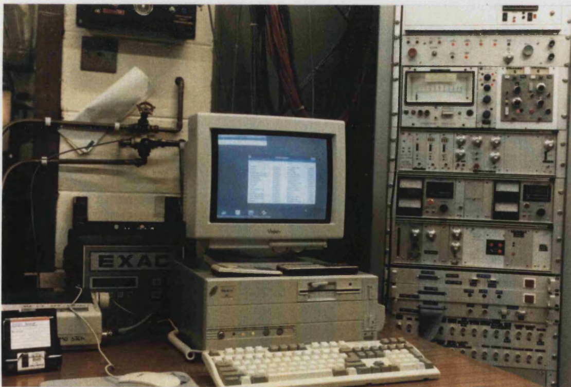
Figure 4.6 The control and acquisition system for the TL-11 test cell
