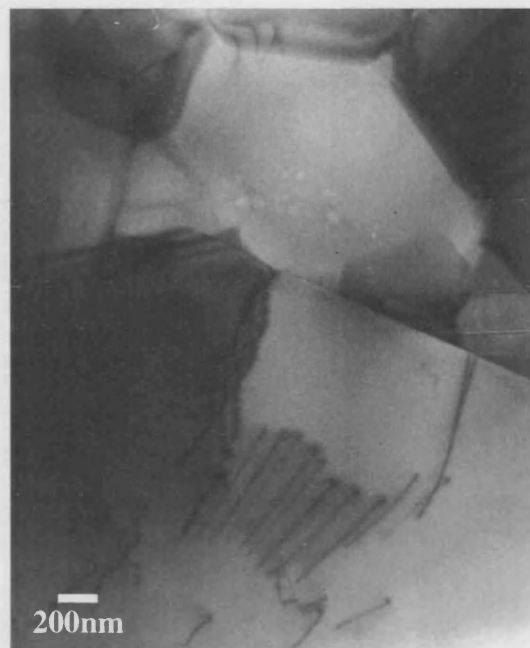
Figure 5.52: Dislocations in the grains in Base composition
